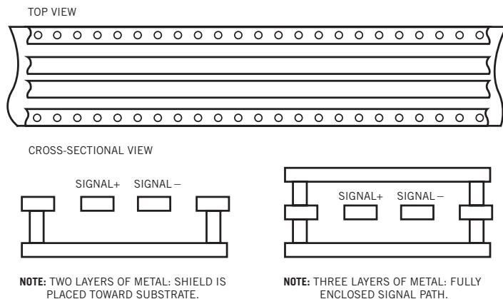
**NOTE:** TWO LAYERS OF METAL: SHIELD IS PLACED TOWARD SUBSTRATE.
