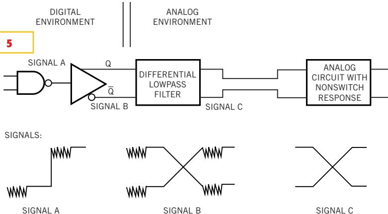
**You can pass digital control into an analog environment with minimal noise effects.**
