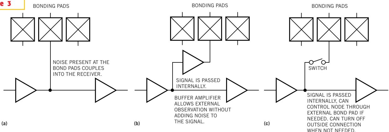
**Avoiding off-chip noise coupling:** You can connect signals to an external pin, but this approach causes signal noise (a). In another approach, you can pass the signal internally and use a buffer amplifier to allow external observation (b). Another approach allows external observation and the ability to connect to the internal node (c). Digital control allows isolation from external noise if the pin is not in use.
